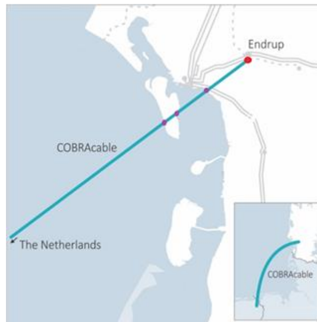
Figure 28 Route of the COBRACable on the Danish side [78]
