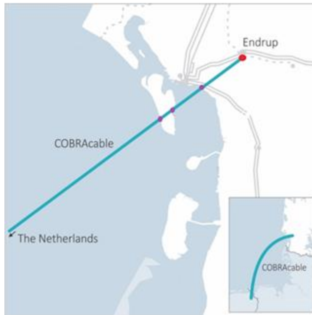
Figure 3: Map of the COBRACable at the Danish side [2]
