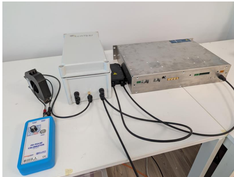
Figure 17. Integrated PD interrogator and PD sensor.
